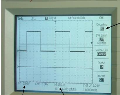
Use '**DC coupling**' – if you use '**AC coupling**' you will not be able to measure absolute voltage levels, i.e., do we have voltage levels representing 1s or 0s.
